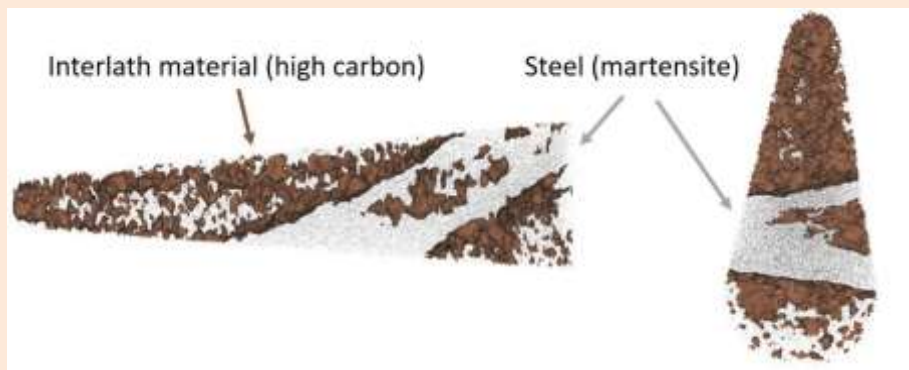
Laser-assisted atom probe tomography of weld region showing carbon and steel composition.
